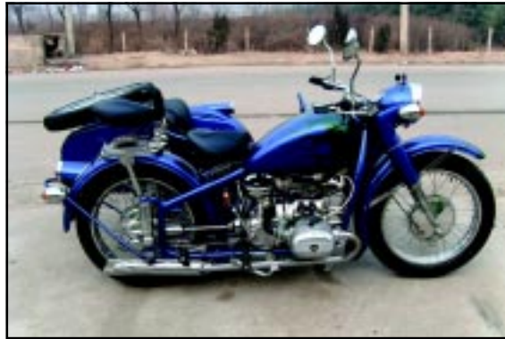
The engine is a 750cc twin cylinder boxer.
