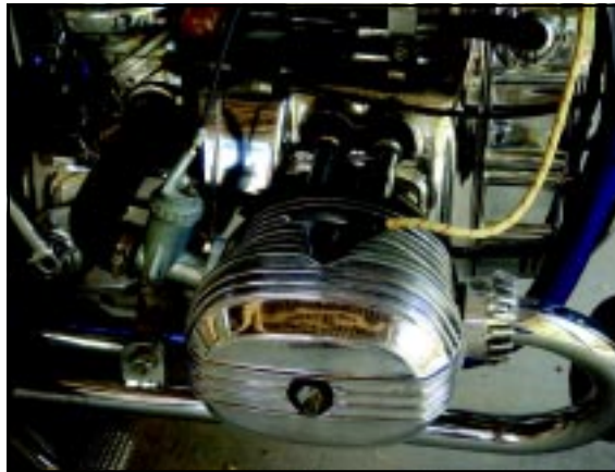
The engine is a 750cc twin cylinder boxer.
